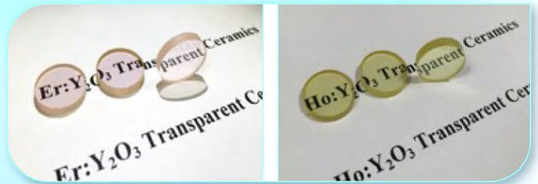
Samples of the fabricated laser ceramics
