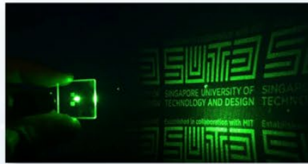
3D printed hologram with nanoscopic elements.
