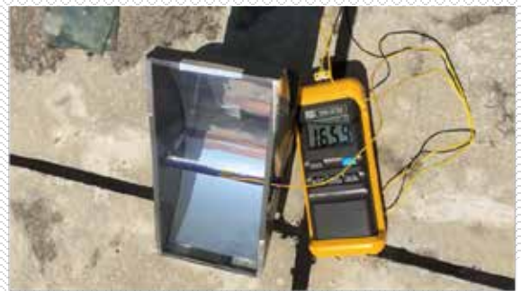
Figure 2. Demonstration of heating performance of our solar absorber under sun light. ~ 160 °C is reached after exposure to sun light for 15 min.
